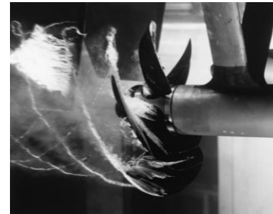
Figure 5. Cavitation at the propeller blade tips in a water tunnel test.
